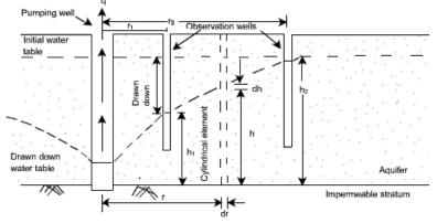
In this test, the pumping causes a drawdown in an unconfined (i.e. open surface) soil stratum, and generates a radial flow of water towards the pumping well. The steady-state heads  $h_1$  and  $h_2$  in observation wells at radii  $r_1$  and  $r_2$  are monitored till the flow rate **q** becomes steady.
