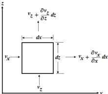
Velocity at the inlet face in the horizontal direction =  $v_x$ Velocity at the inlet face in the vertical direction =  $v_z$ Velocity at the outlet face in the horizontal direction =  $v_x + \frac{\partial v_x}{\partial x} \cdot dx$ Velocity at the outlet face in the vertical direction =  $\frac{\partial v_x}{\partial x} dx$  Velocity at the outlet face in the vertical direction =
