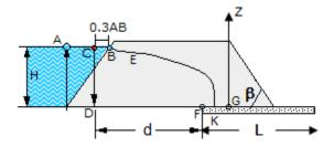
7. Let the distance between focus, F, and directrix, G, be S. i.e., S = 2pThe quantity of seepage per unit length of earth dam with toe filter is q = kS = k x (2 x p) = 2kp
