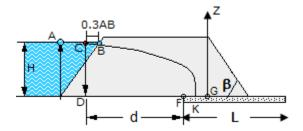
6. Upstream Correction: Sketch the section BE such that it is normal to the upstream sloping surface (i.e. equipotential line). BEK is the phreatic line (top flow line)
