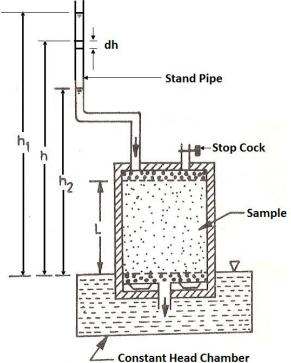
Consider the instant when the head is h. For the infinitesimal small time dt, the head falls by dh. Let the discharge through the sample be q. Let the cross-sectional area of the standpipe be a. From the continuity of flow,
