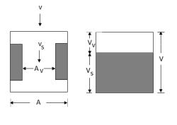
A relationship between the discharge velocity and the seepage velocity can be established referring to the figure, where a longitudinal section through a sample of soil in which the voids and solid particles are segregated.
