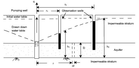
Artesian conditions can exist in а aquifer of thickness **D** confined both above and below by impermeable strata. In this, the drawdown water table is above the upper surface of the aquifer.
